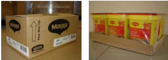
The original carton format (left) and the new Eurotainer with shrink film (right)
